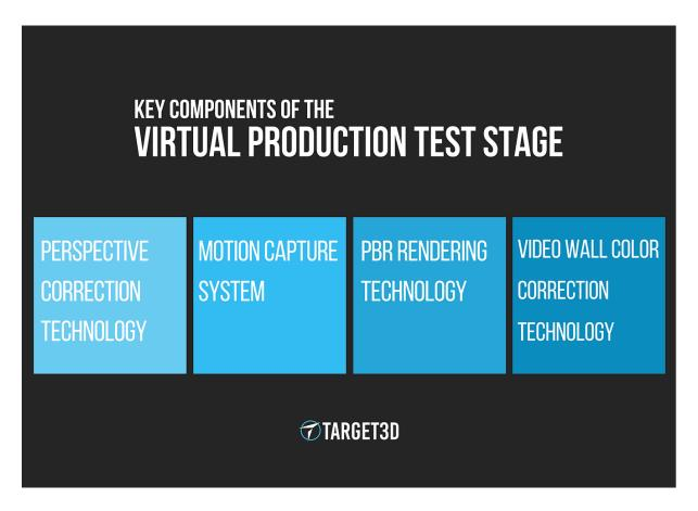
**PERSPECTIVE CORRECTION TECHNOLOGY** calculates and corrects the spatial position and viewing angle of the screen to ensure the correct perspective and parallax is achieved by calculating the relationship between the screen and the live action camera. The performer and camera are free to move around the stage, whilst the digital world is processed from the right perspective and applied to the video screens in real-time - ensuring the final image always looks correct.
